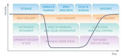
CRAYVALLAC® rheology modifiers provide coatings with a high viscosity under the low shear conditions which are typical of storage, resulting in excellent anti-sedimentation characteristics in pigmented systems thus maintaining a good dispersion and preventing hard settling.
