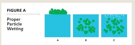
A. Dry solids added to aqueous solution of additives/dispersants require a reduced surface tension to properly wet the surface. Faster wetting = faster process.
