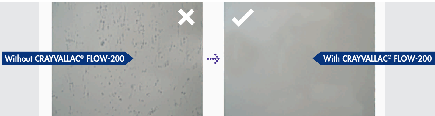
EXAMPLE OF COIL COATING WITH AND WITHOUT CRAYVALLAC® FLOW-200
