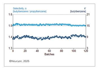
HPLC offers high consistency and reproducibility, which is essential for regulated industries like pharmaceuticals. Kromasil<sup>®</sup> stationary phases have demonstrated excellent batch-to-batch consistency over the years.
