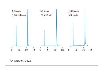
Kromasil's<sup>®</sup> HPLC medias high throughput and efficiency enable fast processing of large material volumes, crucial for industrial-scale production without compromising separation quality. Additionally, prep HPLC offers smooth scalability, allowing methods developed on a smaller scale to be easily scaled up for full production, with consistent results across different particle sizes
